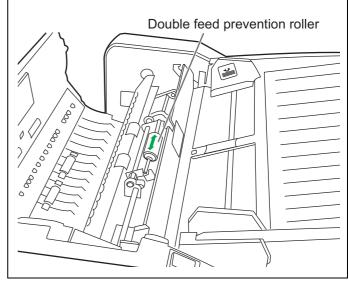
6 Close the double feed prevention conveyor in the direction of the arrow shown in the figure.
